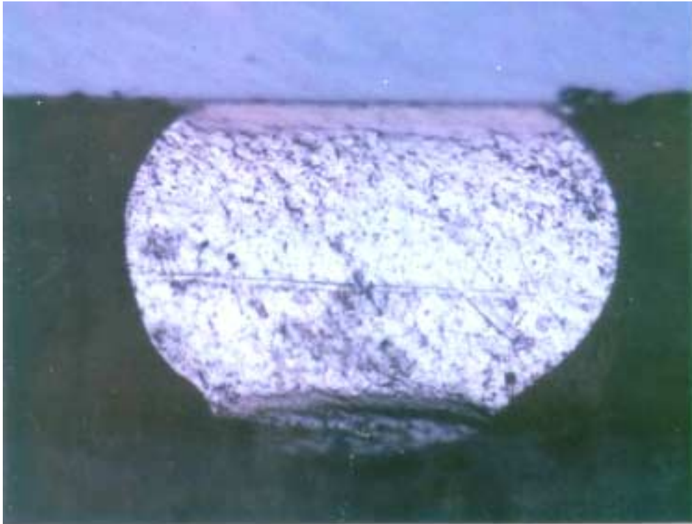
Figure 3. Eutectic solder bump with solder clad finish. Bonding force: 20N
