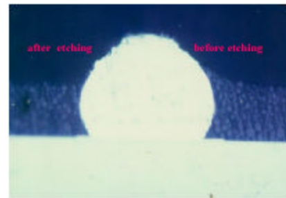
Fig. 8 Cross-section image of a coated wafer bump before and after laser etching
