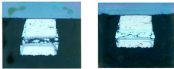
Figure 8. Cross-section images of pillar bump after TCT 1000 cycles (a) pre-reflow (b) non-reflow
